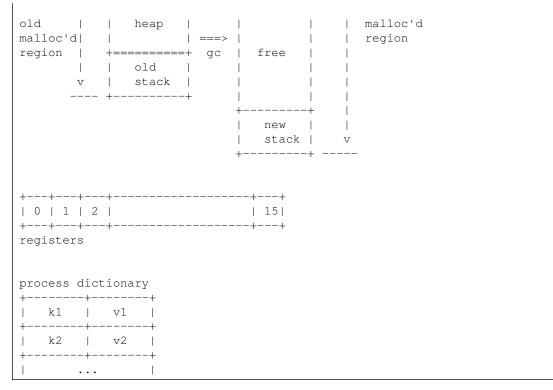
Terms stored in the stack, registers, and process dictionary are either single-word terms (like atoms or pids) or term references, i.e., single-word terms that point to boxed terms or list cells in the heap. These terms constitute the "roots" of the memory graph of all "reachable" terms in the process.
