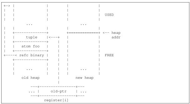
The boxed term is copied to the new heap, overwritten with the marked header 0x2b, along with a pointer to the new term, and the root term is updated with the same address:
