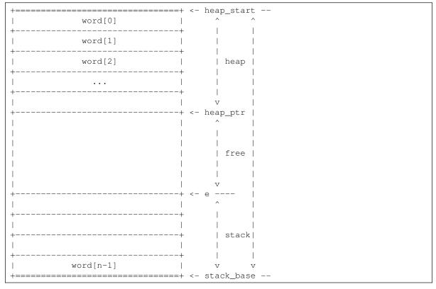
The initial size of the allocated block for the stack and heap in AtomVM is 8 words. As heap and stack allocations grow, eventually, the amount of free space will decrease to the point where a garbage collection is required. In this case, a new but larger block of memory is allocated by the AtomVM OS process, and terms are copied from the old stack and heap to the new stack and heap. Garbage collection is described in more detail below.
