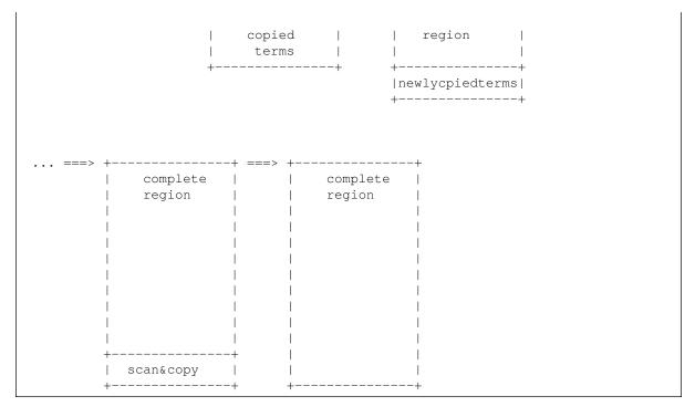
At the end of the iterative scan and copy, all reachable terms in the old heap will be copied to the new heap, and no boxed terms in the old heap will contain pointers to terms in the old heap. Any terms that have not been copied to the new heap are "garbage", as there are no longer any paths to them from the root set, and can therefore be destroyed,
