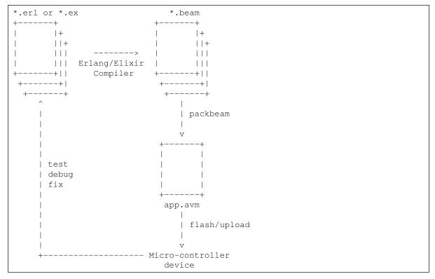
The typical compile-test-debug cycle can be summarized in the following steps:
