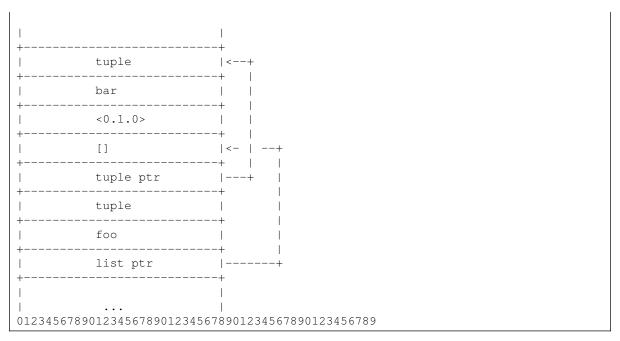
The tuple {bar, self()} is allocated in a block, and the list [{bar, self()}] (or, technically, [{bar, self()} | []]) contains elements that *point* to it elements (in this case, [] and {bar, self()} – note that in general, in AtomVM, the address of the tail of a list occupies the first byte in the list – more details on that below). Finally, the tuple {foo, [{bar, self()}]} contains the atom foo and a *pointer* to the list it contains.
