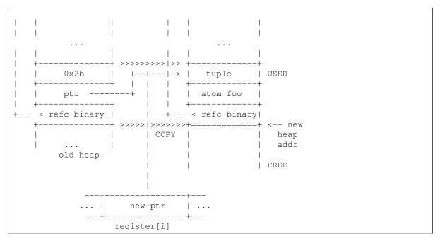
Note that the first term of the tuple (atom foo) is copied to the new heap, but the pointer to the refc binary is out of date – it still points to a value in the old heap. This will be corrected in the iterative scan and copy phase, below.
