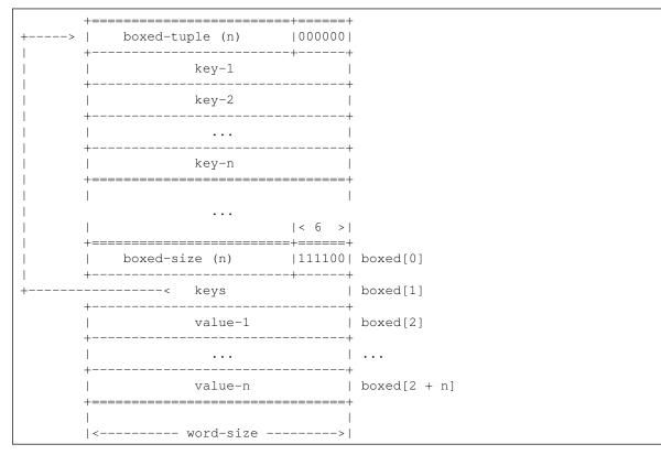
The tuple of keys may or may not be contiguous with the boxed term holding the map itself (and in general will not be, after garbage collection). In addition, maps that are modified [sic] via the := operator (or via =>, when the key already exists in the source map) share the keys tuple, for space efficiency.
